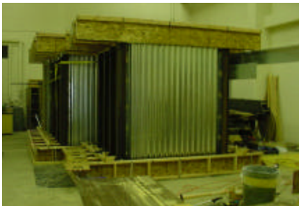
Side Elevation of the Steel Deck Shear Wall with Steel Boundary Columns
