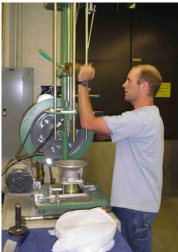
Undergraduate student Tyler Young compacts a cement-treated specimen in the laboratory.
